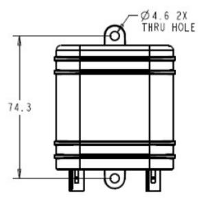
Figure 3: Mounting dimensions of a GPS-201/202
