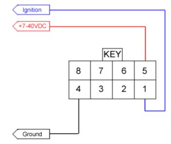
Figure 5: Wiring for Power Only (HRNSxx)
