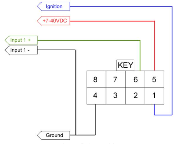
Figure 7: Wiring for Power and I/O
